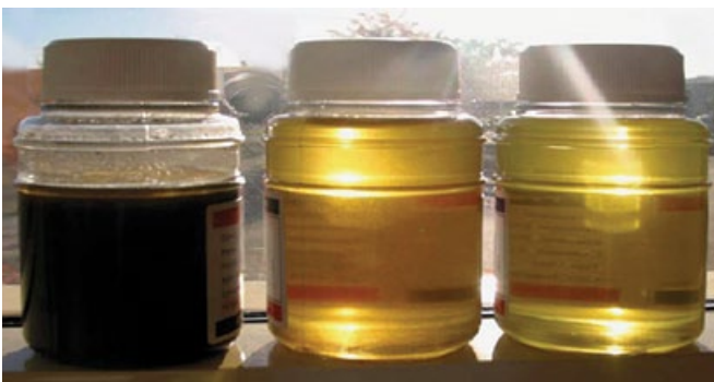
Left - Right Oil entering the filter unit; oil after 8 hrs filtering; filtered oil re-entering the fryer
