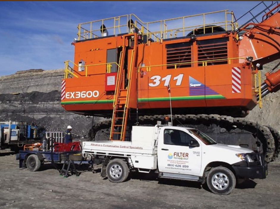
Trailer mounted units enable kidney loop filtration to be carried out in-situ
