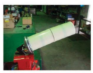
Purpose designed specifically for use in the element change procedure when servicing all Filter Technology Australia filter systems.
