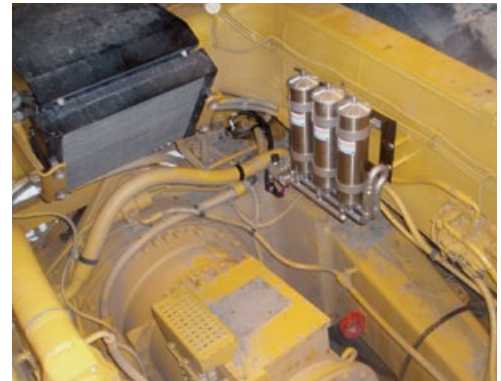
Onboard filtration system fits neatly in chassis, with plenty of access for filter changes.
