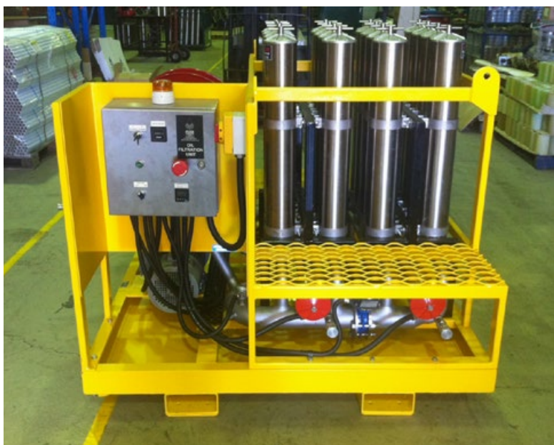
FM41646 filtration unit - custom built version with hoses and hose reels.
